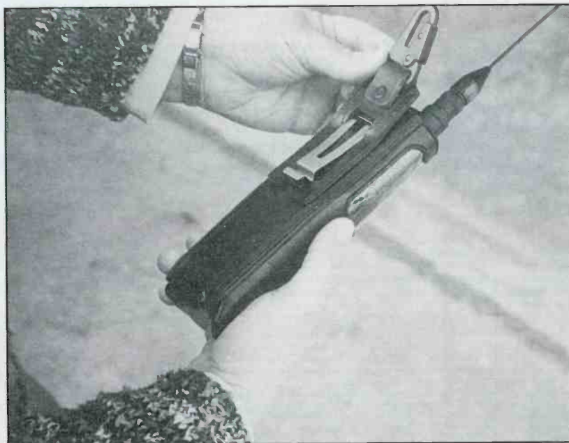
A perfect fit — the Pager Keeper slides over the Alinco belt clip.
