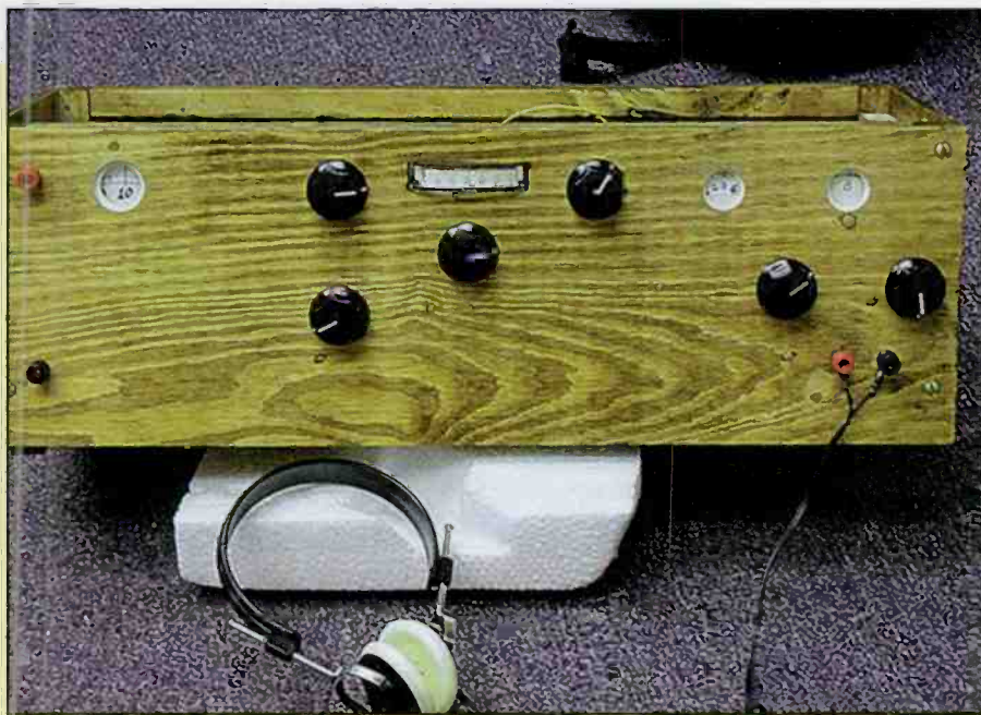
The front panel of George Hawkin's version of the Lyonodyne selective crystal set. Note the three dial scales visible through the portholes showing the logging scales for the antenna tuning capacitor, the coupling position of the wave-trap coil, and the wave-trap tuning capacitor.
