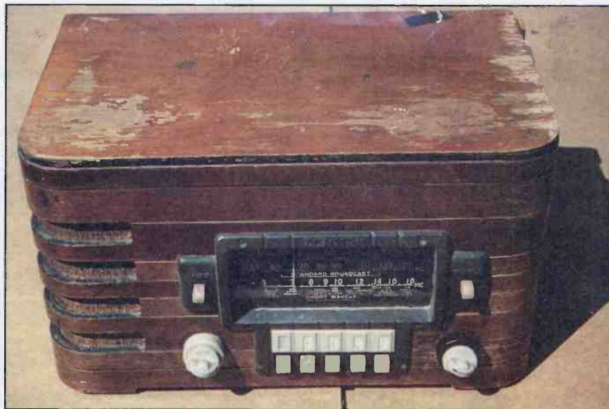
This Zenith table radio contained an unwelcome surprise. An asbestos sheet was placed beneath the cabinet top to deflect the large amounts of heat released by the tube circuitry.
